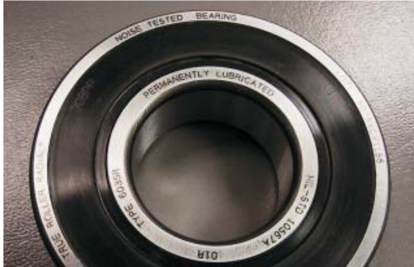
High contrast marking on bearing housings.
